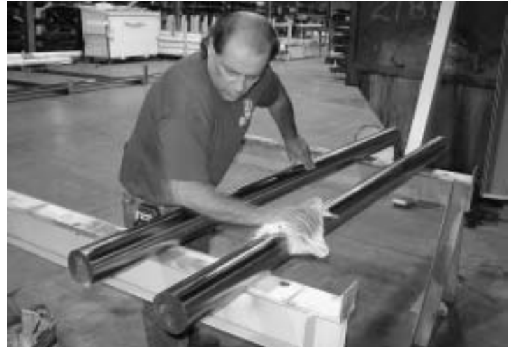
PRECISION FINISH – “NEAR” BEARING FIT
