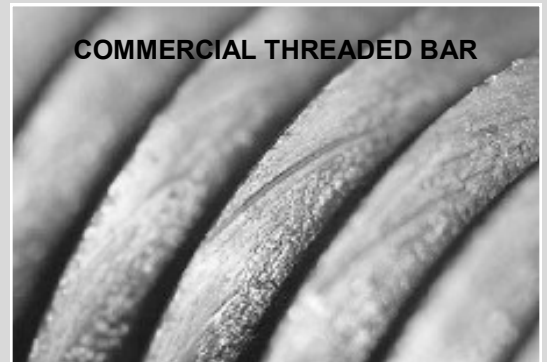
Sharp cuts and gouges, weaken threads and can serve as stress risers.
