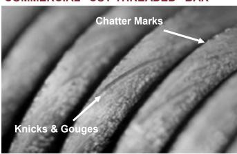
Sharp cuts, with knicks and gouges, weaken threads are stress risers, which will lead to surface initiated fatigue failures. The above macro photograph clearly shows chatter marks and other imperfections.
