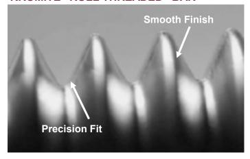
Grain structure is re-defined into continuous unbroken lines. The grain follows the thread contour, similar to a forged bar. The above macro photograph illustrates the quality of the threads. Smooth contours are free of the knicks and gouges that contribute to failure caused by fatigue.
